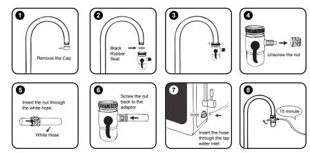
Run a water flow test about 15 minute and your water purifier system are ready to use.
