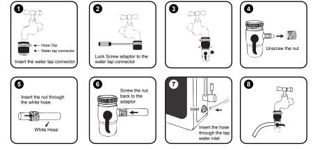
Run a water flow test about 15 minute and your water purifier system are ready to use.
