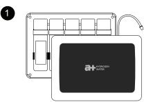
Press left and right clip casing of water system to open the cover of water system
